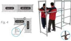
Step 4 | Add an additional unit by connecting two more posts with post connectors and then setting traverses onto the dovetails on the posts. The traverses on the first and second unit share the middle post. Place shelf plates on traverses to complete the second unit. Add an additional unit in a 90° corner using corner connectors. (Fig. 4)
