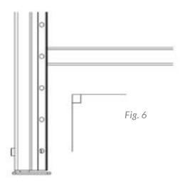
Step 6 | Check that horizontal brace is square to posts before fitting the remainder of the diagonal braces working from the bottom up. (Fig. 6)
