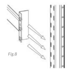
Step 8 | Stand assembled frames in their feet and fit beams at desired heights, starting at the bottom and working up. The connections should slot into posts without force. Once in position they should be hammered in tight with a soft face hammer of reasonable weight. (Fig. 8)
