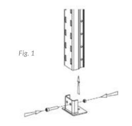
Step 1 | Take two posts and fit the feet with 2 x M8x20 bolt supplied to the bottom of post. The feet may only fit one end of post as hole distance can vary from end to end. (Fig. 1)
