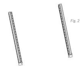
Step 2 | Lay posts parallel at approx desired width of frame (450, 600, 900 etc). (Fig. 2)
