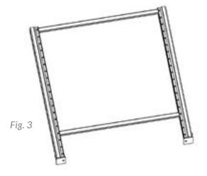
Step 3 | Take two horizontal braces, which will be the shorter of the two supplied, and lay in place at the top and bottom.(Fig. 3)
