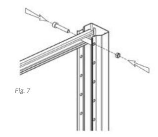
Step 7 | Finish assembly with another horizontal brace with a spacer used on final bolt. (Fig. 7)
