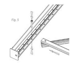
Step 5 | Next, bolt through horizontal and diagonal brace as shown in the drawing (no spacer required). (Fig. 5)
