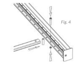
Step 4 | Start by bolting horizontal brace to one post in the 4th hole from the bottom. Use spacer supplied (as shown in drawing). Starting at bottom or foot end. (Fig. 4)
